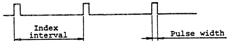
(Fig.315) Typical waveform of TP4 (Speed observation)
