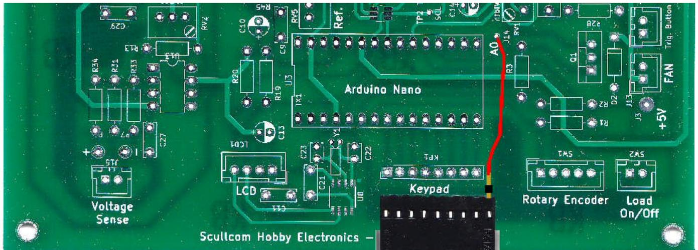
Image show 5th Row connection when using a 5 x 4 Matrix Keypad. Use a single right angled PCB header to connect to the keypad as shown. Connect a wire from that pin to the connection marked A0 on the PCB as shown.
