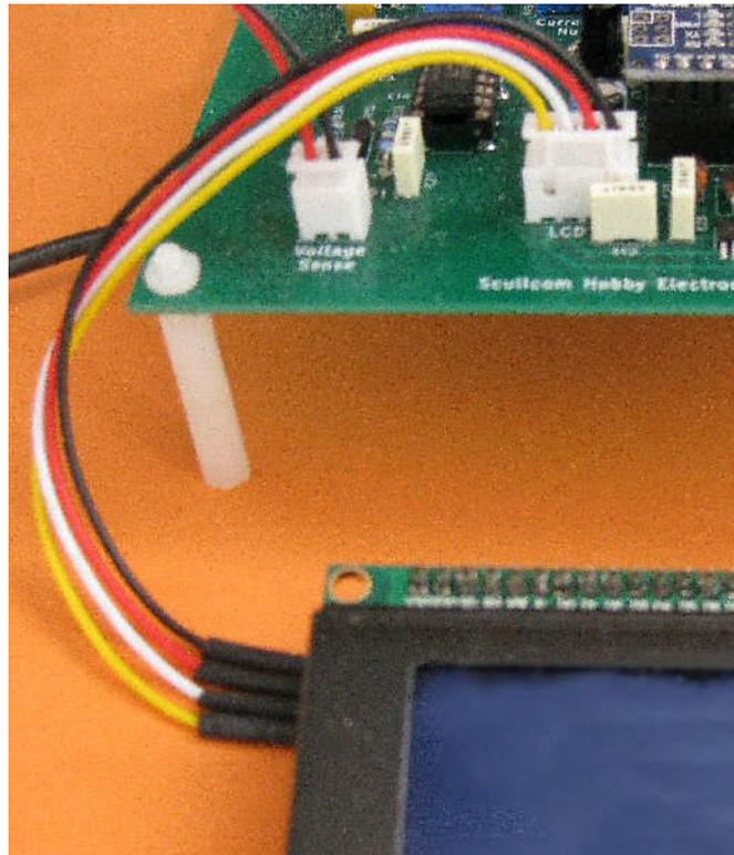
The LCD has an I<sup>2</sup>C module fitted.
