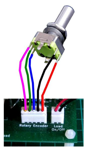
Typical wiring for the Rotary Encoder connections to the PCB socket/plug
